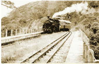
CLIMBING THE BELLEVUE PASS A rare archive photo showed a train climbing Bellevue pass pulled by a Swiss steam locomotive on the first part of the trail that was equipped with a cogwheel track at the point of intersection of Krongkeo-Eo Gio, which also included a siding. This photo was probably taken in the early period of Vietnam War, during which the line was still used daily. Notice that the two-line crossing platform was also equipped with cogwheel track.
